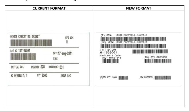
Moisture Sensitivity Level (MSL 3) and Manufacturing Labels to 2-in-1 Label.
