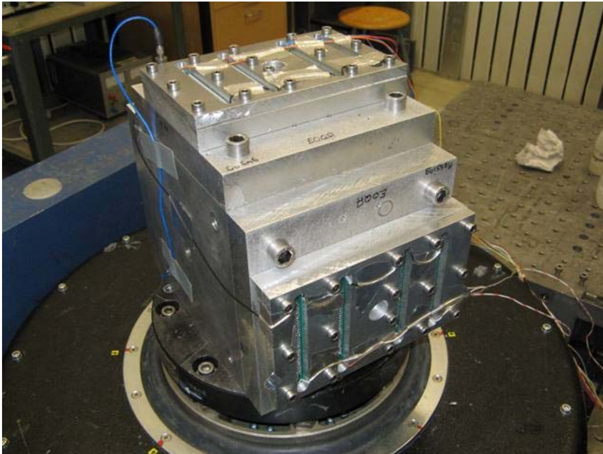
Pic. 1 EUTs mounted on shaker table
