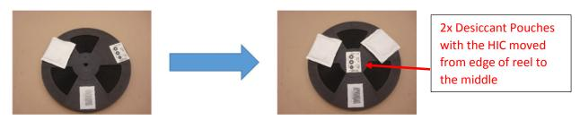
**Additional Note:** Typically, the Moisture Barrier Bag (MBB) is not opened within 10-12 days from the date the bag was sealed and shipped to customers. However, with the addition of another desiccant pouch, they improve the time required for the HIC to turn blue. We are still requesting that the product be opened and inspected a minimum of 10 days post MBB seal date. This is to allow sufficient time for the desiccant to absorb the moisture and the HIC to turn Blue.
