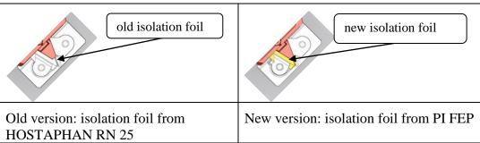
Replacement of isolation foil and improvement of internal bus bars for a more robust design against moisture. Nevertheless climate class 3K3 will not change.
