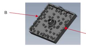
The injection point moves from point "A" to point "B".
