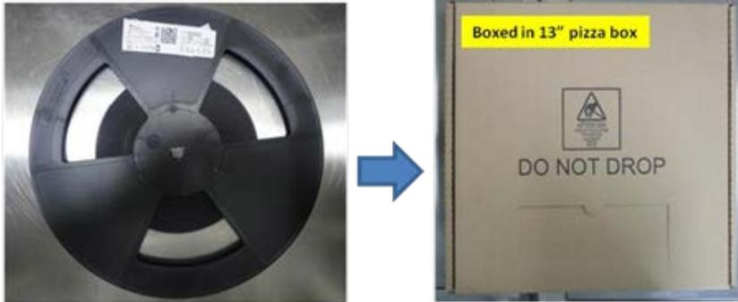
Proposed Packing for full SPQ (3ku) – 7 inch reel diameter
